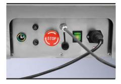
**Emergency stop button** The base has an emergency stop button.
